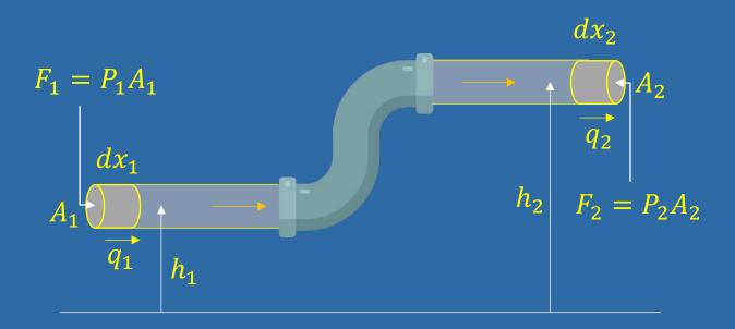
Let us consider a container in the shape of a pipe, whose two edges are placed at *different heights* and varying diameters. The relationship between the areas of cross-sections A, the flow speed q, height from the ground h, and pressure p at two different points 1 and 2 are given in the figure below.
